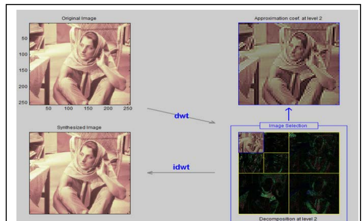
Fig. 13: Displaying the forward DWT and inverse DWT of image, using GUI in MATLAB
